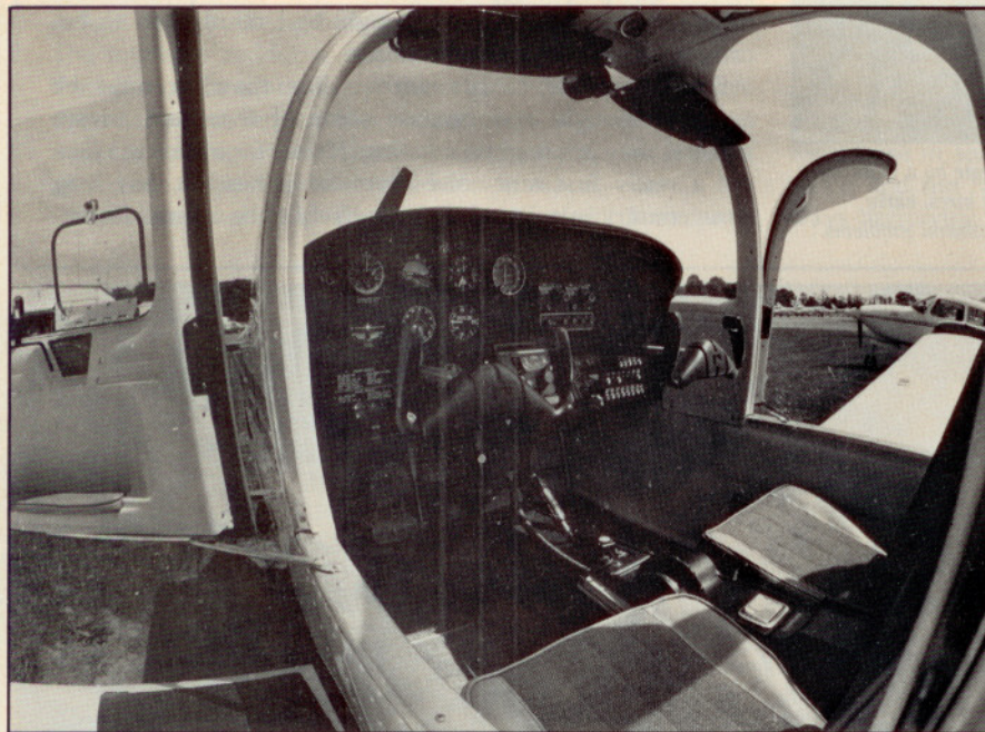
The Tomahawk's cockpit is a classic example of a fine design compromised by manufacturing. With a toolbox, patience, a little money and a lot of time, a diligent owner could reduce the annoyance caused by such things as ill-fitting doors and their induced noise.
